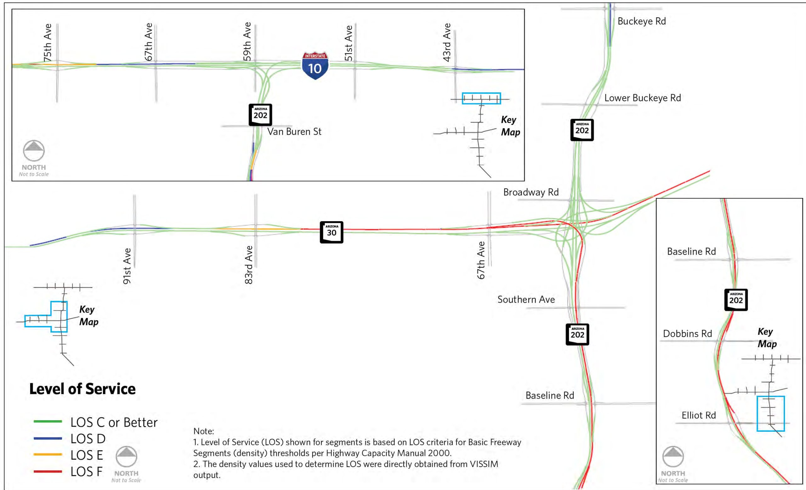
Figure 6.14. SR 30/SR 202L System Traffic Interchange, 2040 PM Peak Hour 3 Level of Service
