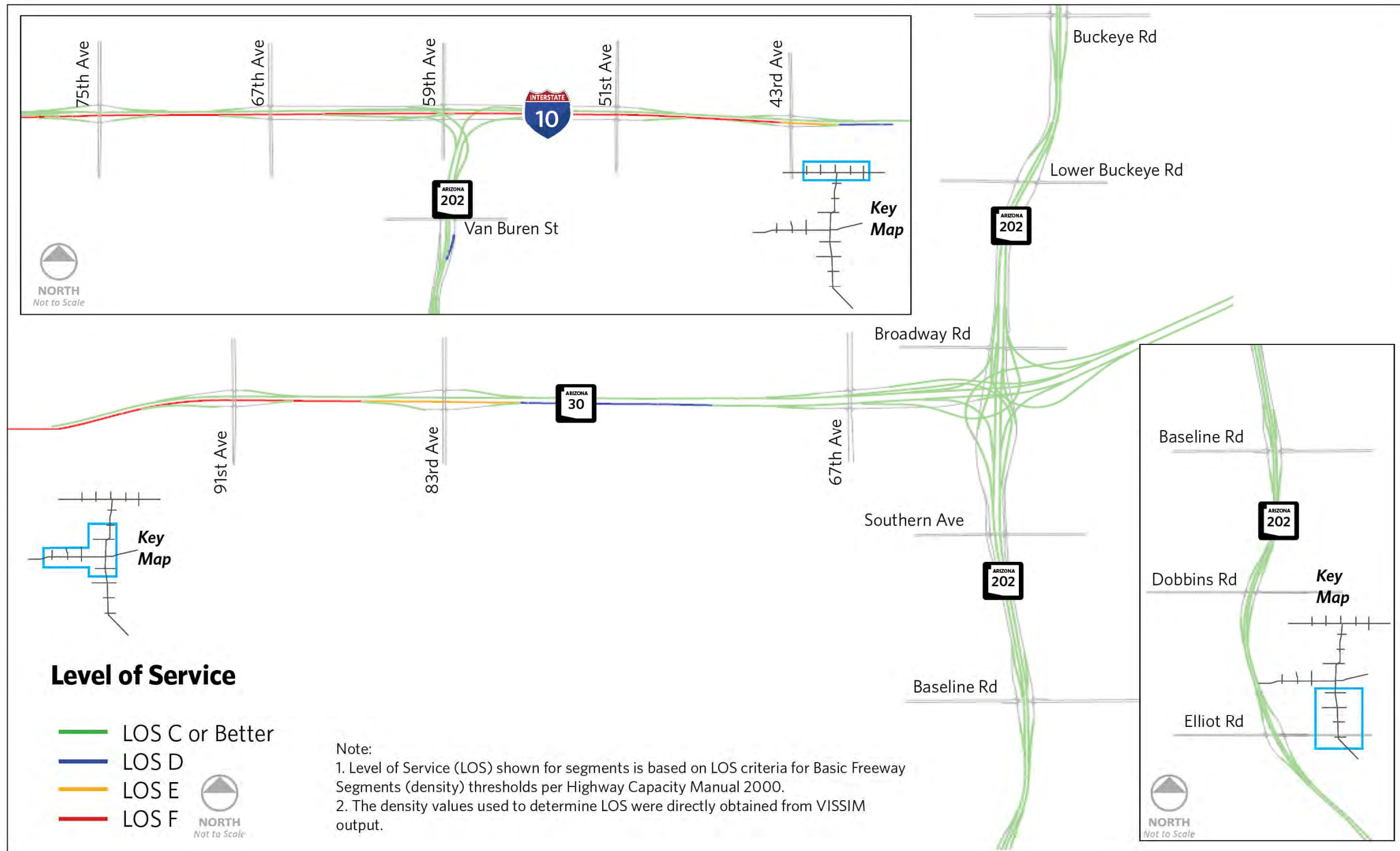
Figure 6.11. SR 30/SR 202L System Traffic Interchange, 2040 AM Peak Hour 3 Level of Service
