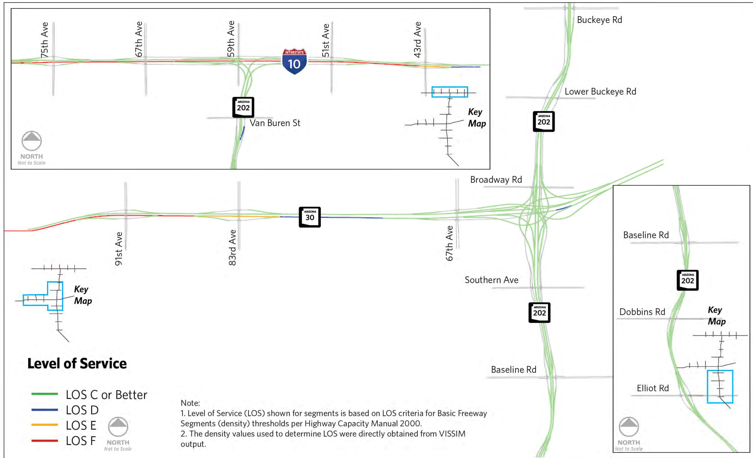
Figure 6.5. SR 30/SR 202L System Traffic Interchange, 2035 AM Peak Hour 3 Level of Service
