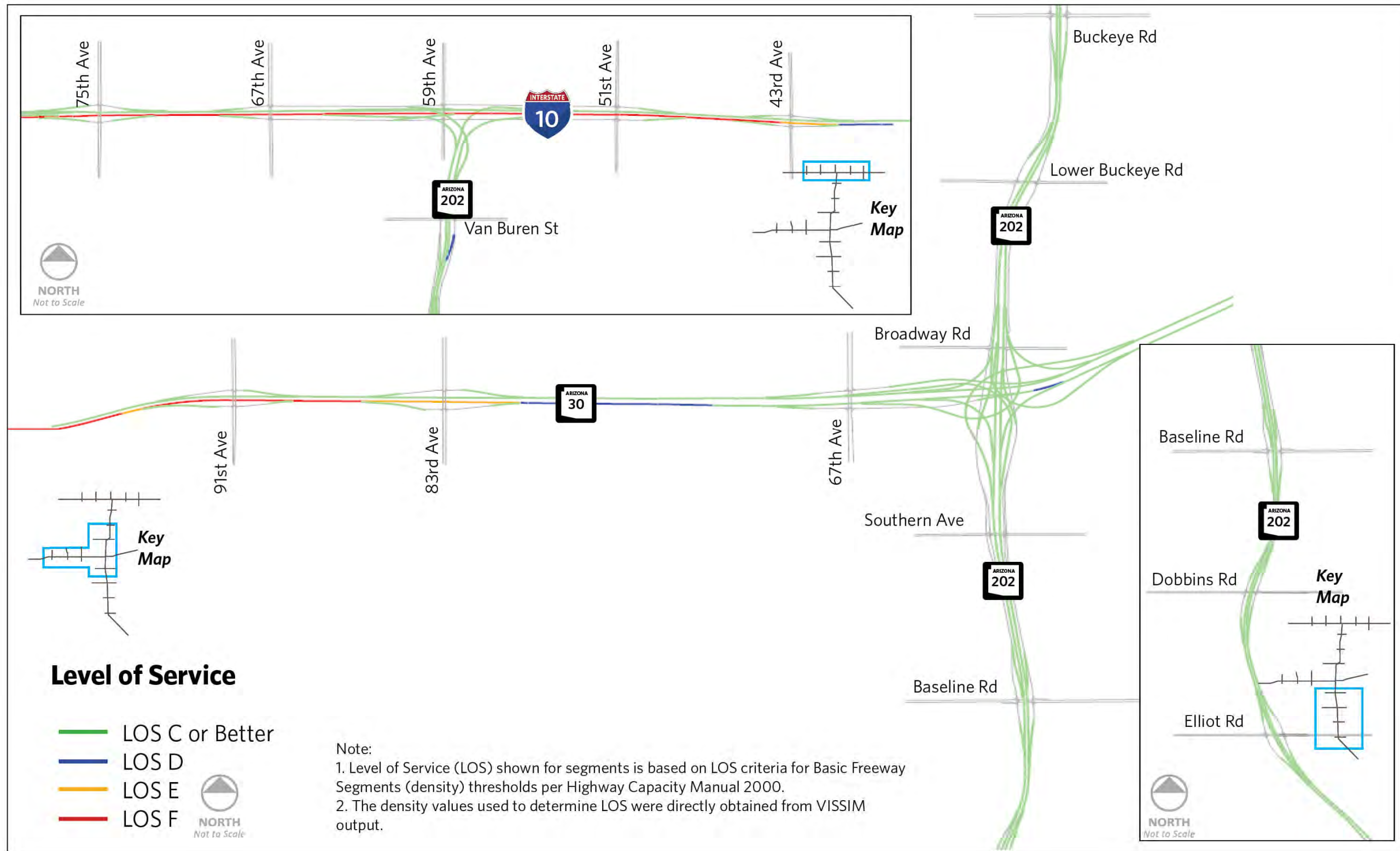
Figure 6.3. SR 30/SR 202L System Traffic Interchange, 2035 AM Peak Hour 1 Level of Service
