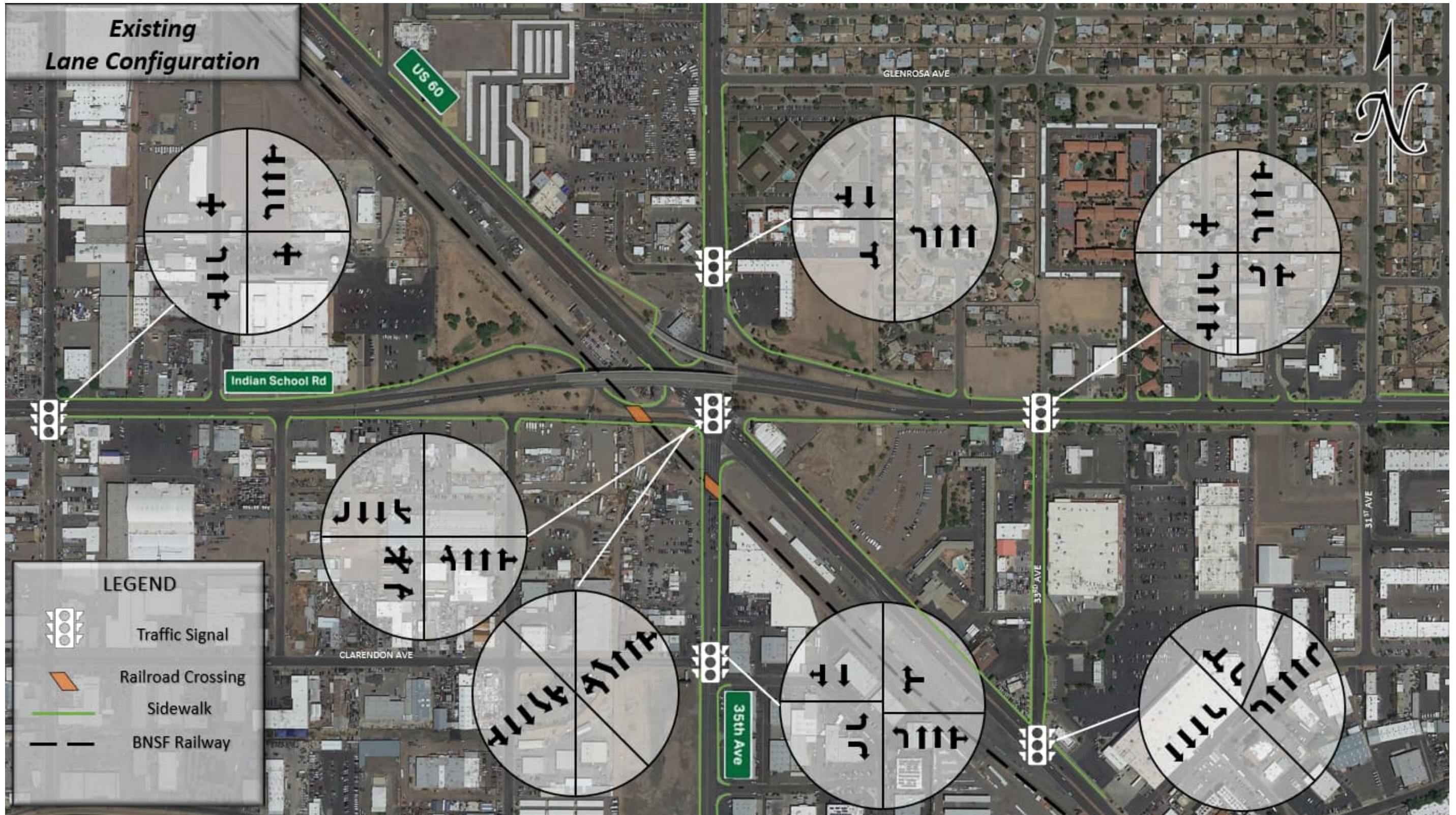
Figure 11 – Existing Lane Configurations
