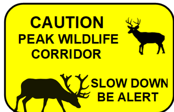
Figure 3-2. Conceptual motorist alert signs at the approaches to a designated Wildlife Collision Prevention Zone; the signs should be LED-enhanced for maximum nighttime impact.
