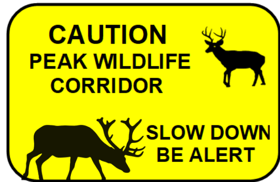
Figure 3- 51. Conceptual layout for motorist alert signs at the approaches to a designated Wildlife Collision Prevention Zone; the signs should be LED-enhanced for maximum nighttime impact.
