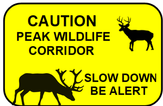
Figure 3- 11. Conceptual layout for motorist alert signs at the approaches to a designated Wildlife Collision Prevention Zone; the signs should be LED-enhanced for maximum nighttime impact.
