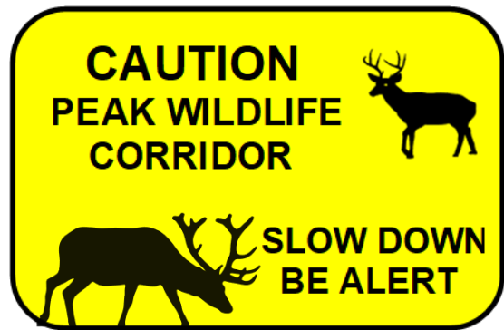
Figure 3- 83. Conceptual motorist alert signs at the approaches to a designated Wildlife Collision Prevention Zone; the signs should be LED-enhanced for maximum nighttime impact.
