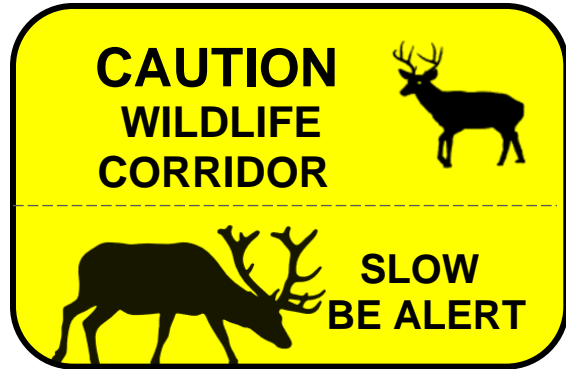
Figure 3- 85. Conceptual fold-down seasonal motorist alert signs at the approaches to a speed reduction zone; signs should be LED-enhanced for maximum nighttime impact.
