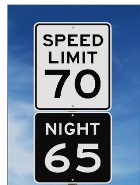
Figure 3- 63. Static stacked daytime/nighttime speed limit signs.
