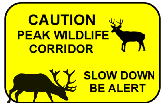
Figure 3- 28. Conceptual layout for motorist alert signs at the approaches to a designated Wildlife Collision Prevention Zone; the signs should be LED-enhanced for maximum nighttime impact.
