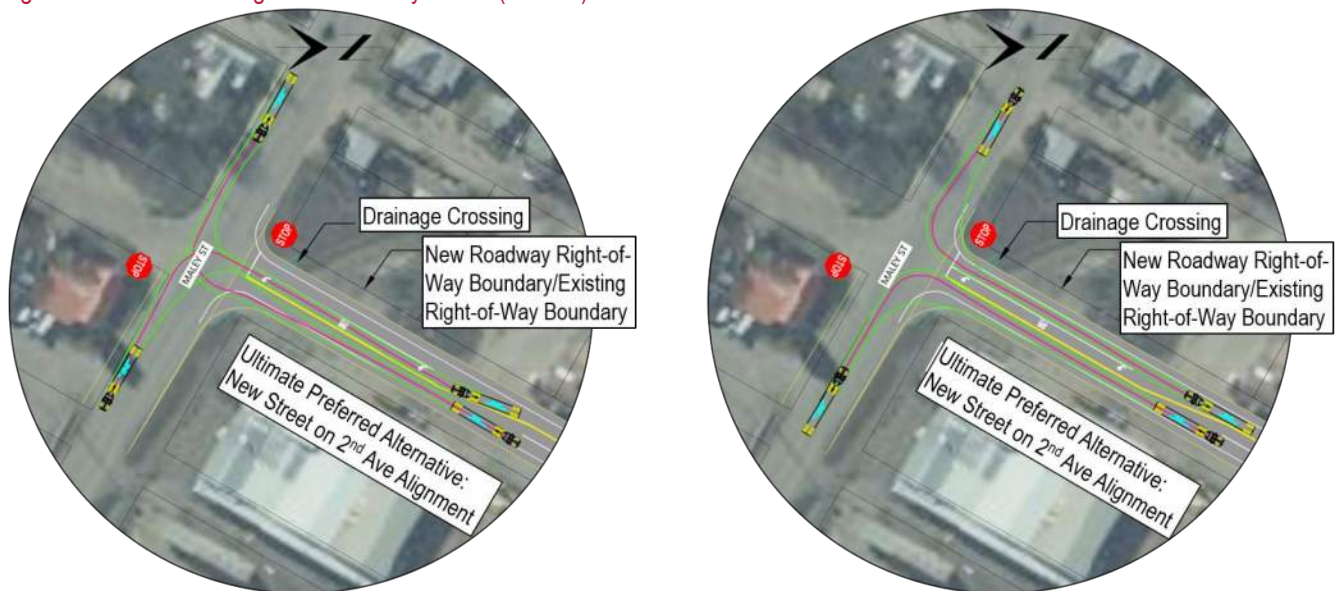
Figure 68. WB-67 Turning Paths at Maley Street (SR 186) and 2 nd Avenue
