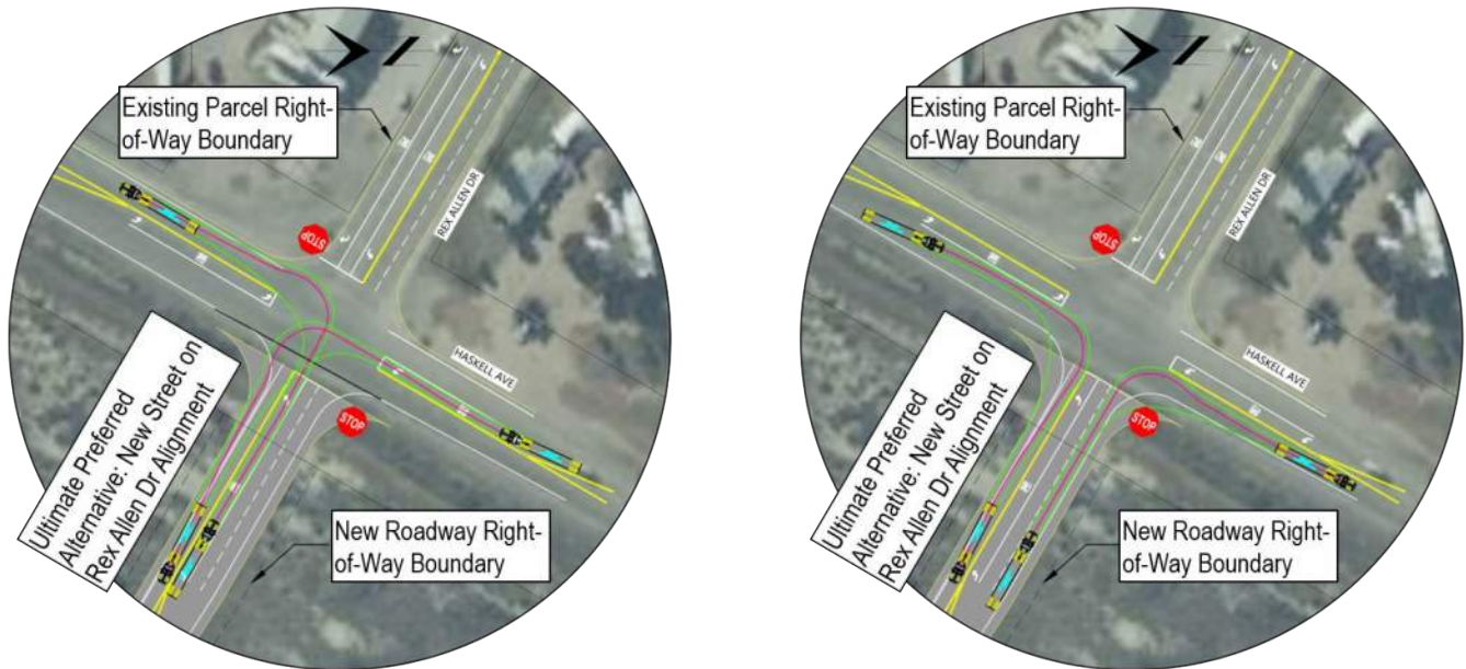
Figure 69. WB-67 Turning Paths at Haskell Avenue (B-10) and Rex Allen Drive (SR 186)
